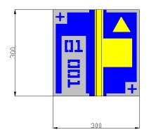
All dimensions in microns Chip thickness 100 µm Polarity: p-contact (anode) up
