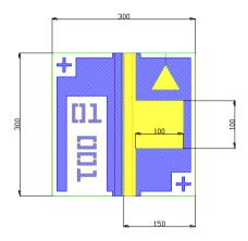
All dimensions in microns Chip thickness 100  $\mu$ m  $\pm$  10  $\mu$ m Polarity: p-contact (anode) up
