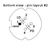
All dimensions are millimeters (mm). The default pin layout is #2 (shown). Other pin layouts are available as per customer request. Monitoring photodiode is optional, not included by default.
