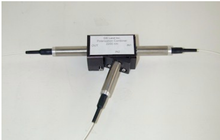
Figure 1. Free space optics based fiber polarization combiner
