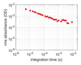
Allan deviation as function of integration time. Only a single spectral element (data point in the spectrum) is considered. Even better results can be achieved on broad absorption features extending over multiple data points.
